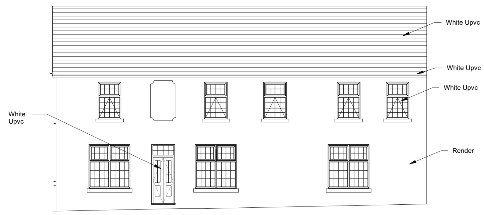
Existing Front Elevation
